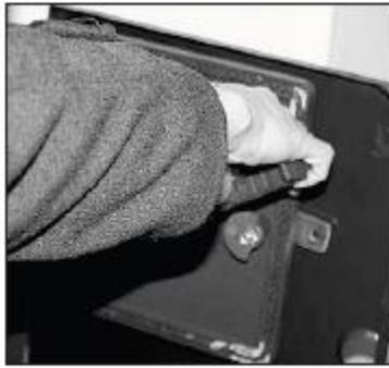
**Fig. 2 Opening the door for stoking**
