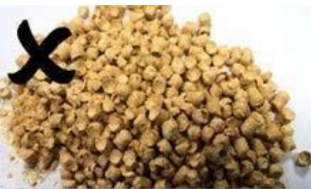
Pellets too short in length
