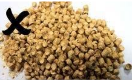
Pellets too short in length
